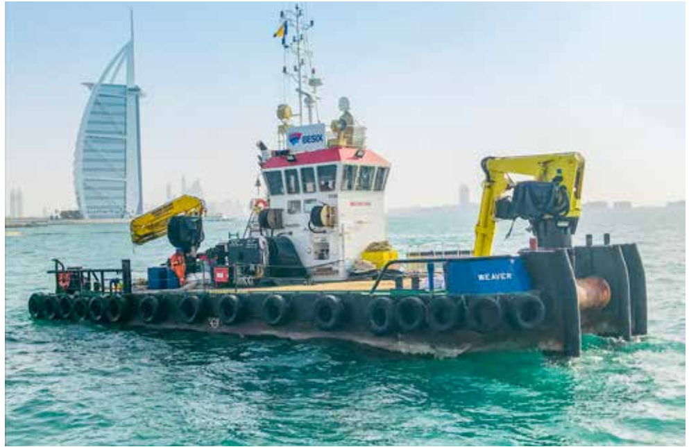
NEW WORK BOAT 'WEAVER' with a 24 tonnes bollard pull capacity, used for moving large size barges and anchor handling
