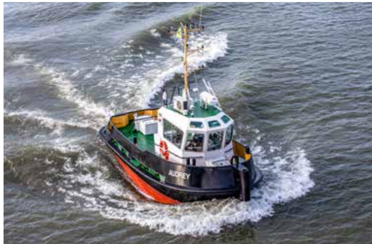
NEW TUG BOAT 'AUDREY' : a medium size assistant tug with 10 tonnes bollard pull capacity
